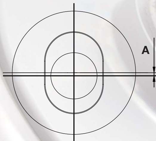
Eccentric hole on bushing
